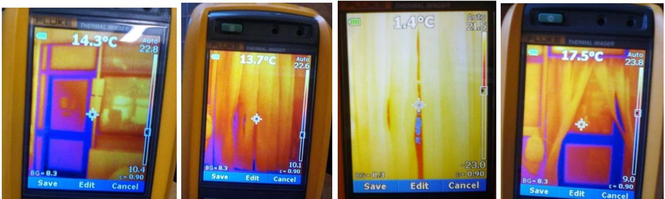
Some classrooms have plastic flaps to help keep the heat in when the door is open. The image on the left shows a door with no insulation. The next image shows a door that was closed with the plastic strips covering the door, the third image is the door open but the strips closed, and the image on the right shows a door closed with the strips pulled back.
